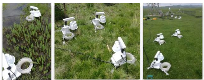
Zoige Wetland Ecosystem by Wetland Research Institute Chinese Academy of Forestry CH 4 /CO 2 /H 2 O Soil Flux System
