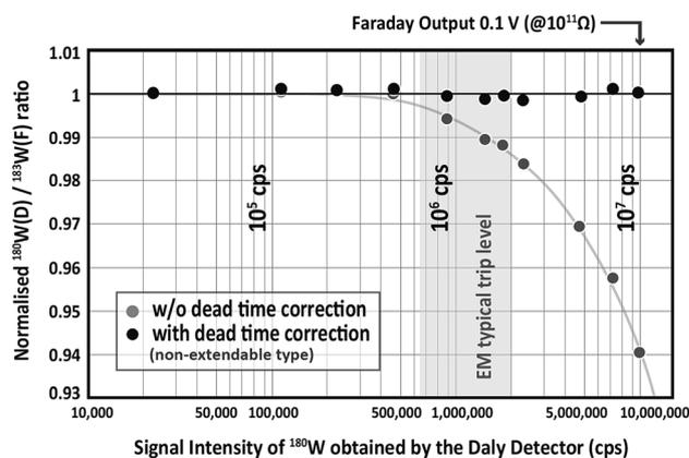
Fig. 2 Measured  $^{180}\text{W}(\text{D})/^{183}\text{W}(\text{F})$  ratio with and without the correction of the counting loss due to the dead time. The gray circles denote the measured signal intensity data without the correction of the dead time, and the black solid circles represent the data after the correction based on the non-extendable model.
